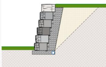
MUR RENFORCE AVEC REMBLAI BETON EN PIEDS
